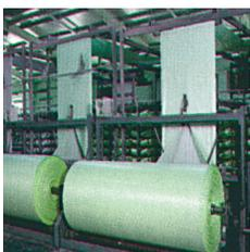
Cut straight of tubular cloth with heating cutter, then winds it to flat cloth.
