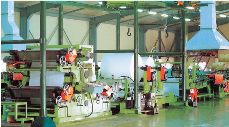
Especially designed to convert Plastic (PP/HDPE) Woven Cloth Roll is to the center-pasted flush cut and notch tubes.
