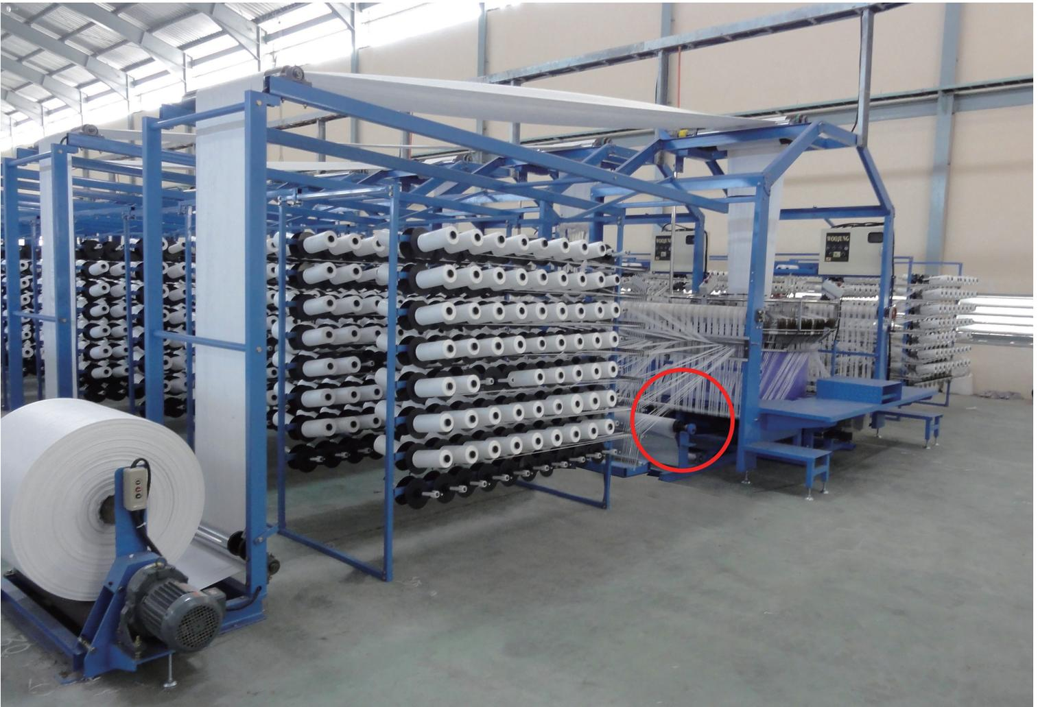
This loom is specially designed to insert 2-layer blown film while weaving tubular cloth.
