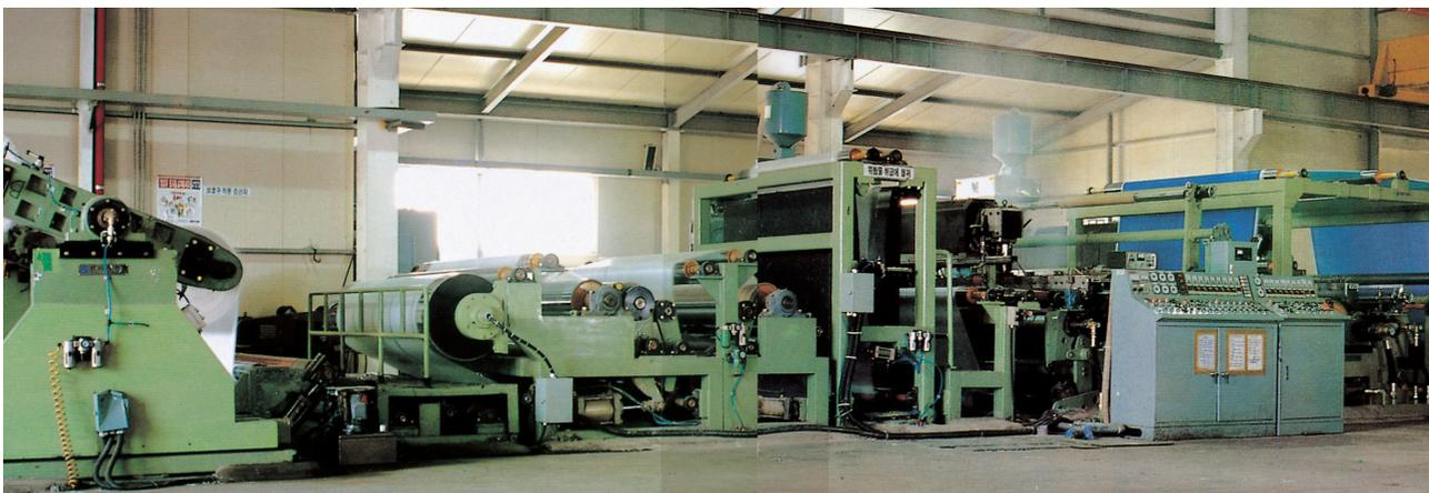
This machine is a tarpaulin coating machine consisting of a single side coating machine, a tandem machine for coating double sides at the same time, and a turning bar system for coating tubular corn bags.
