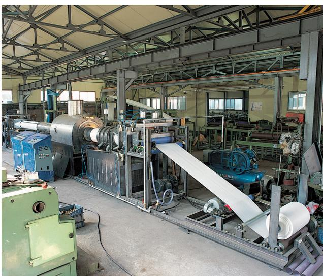
This machine is designed for producing P.P woven inside laminating bags by hot pressure air and air cooling system which is used for water-proof bags such as packing for sugar, chemicals, flour, fertilizer and so on.
