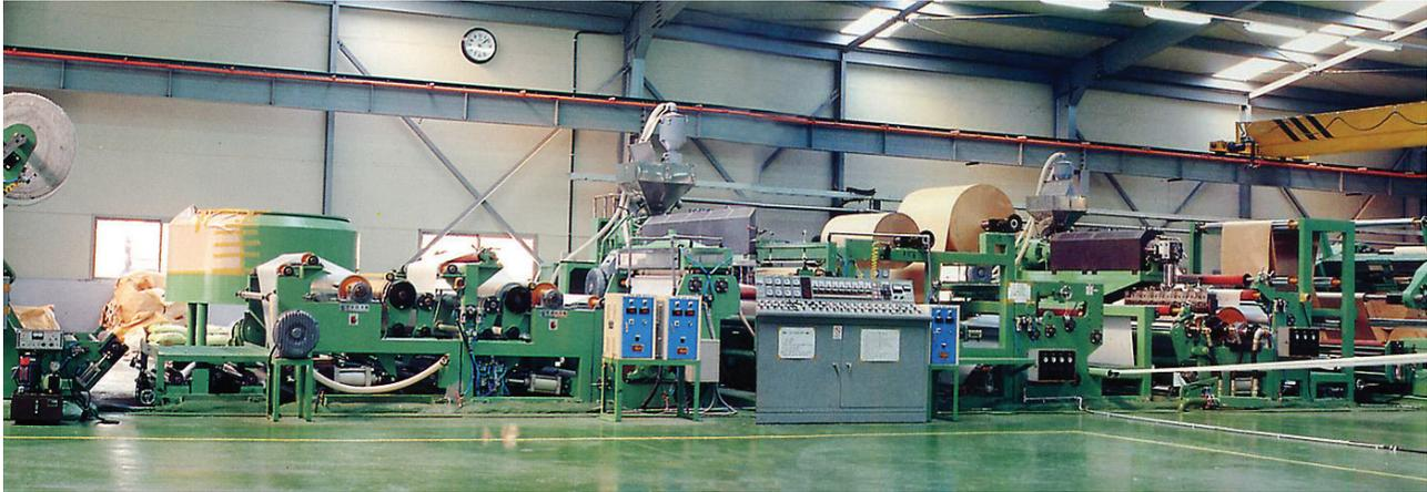
This machine is designed to produce cloths for packages such as cement bag and material bag, by coating P.P or P.E woven cloths or laminating kraft paper.
